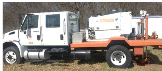
(b) Small-capacity shaker named Thumper that is used to continuously evaluate G_{max} .
