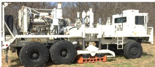
(a) Moderate-capacity shaker named Rattler that is used to create nonlinear soil behavior.
